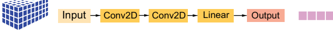
Fig. 7: Deep Neural Network diagram. Final layer is often a Linear (FC) layer in order to map to a probability vector.
